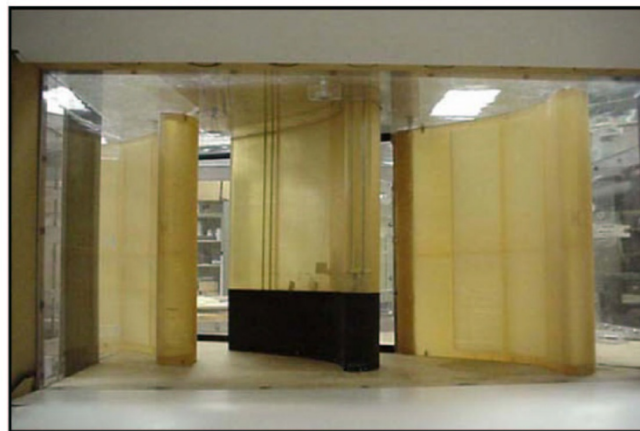
Figure 3. Large-scale turbine blade in wind tunnel.
